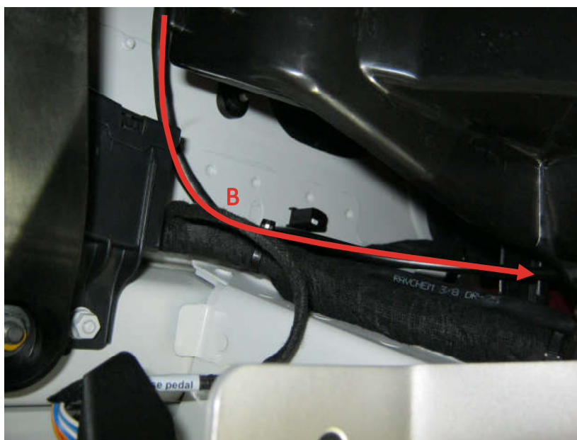
Step 14: Laying the wire harness in the interior (transmission hump direction)
