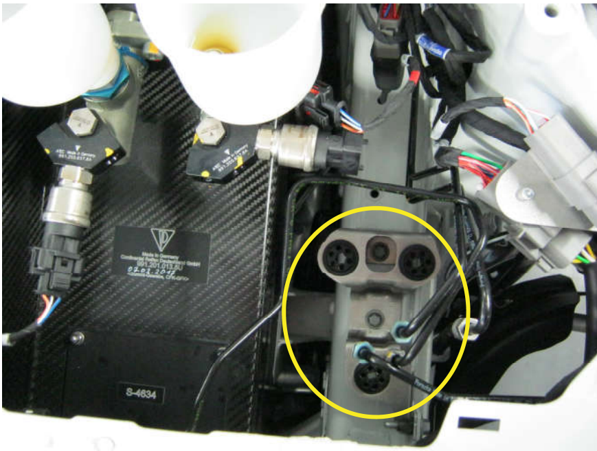
Step 6: The line distributor has been dismantled
