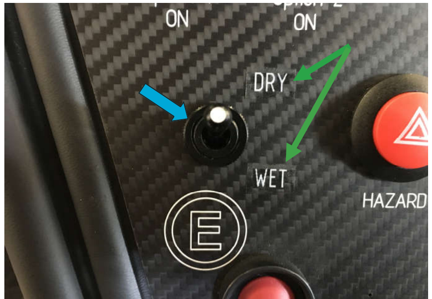
Step 22: Installation of wet-dry switch
