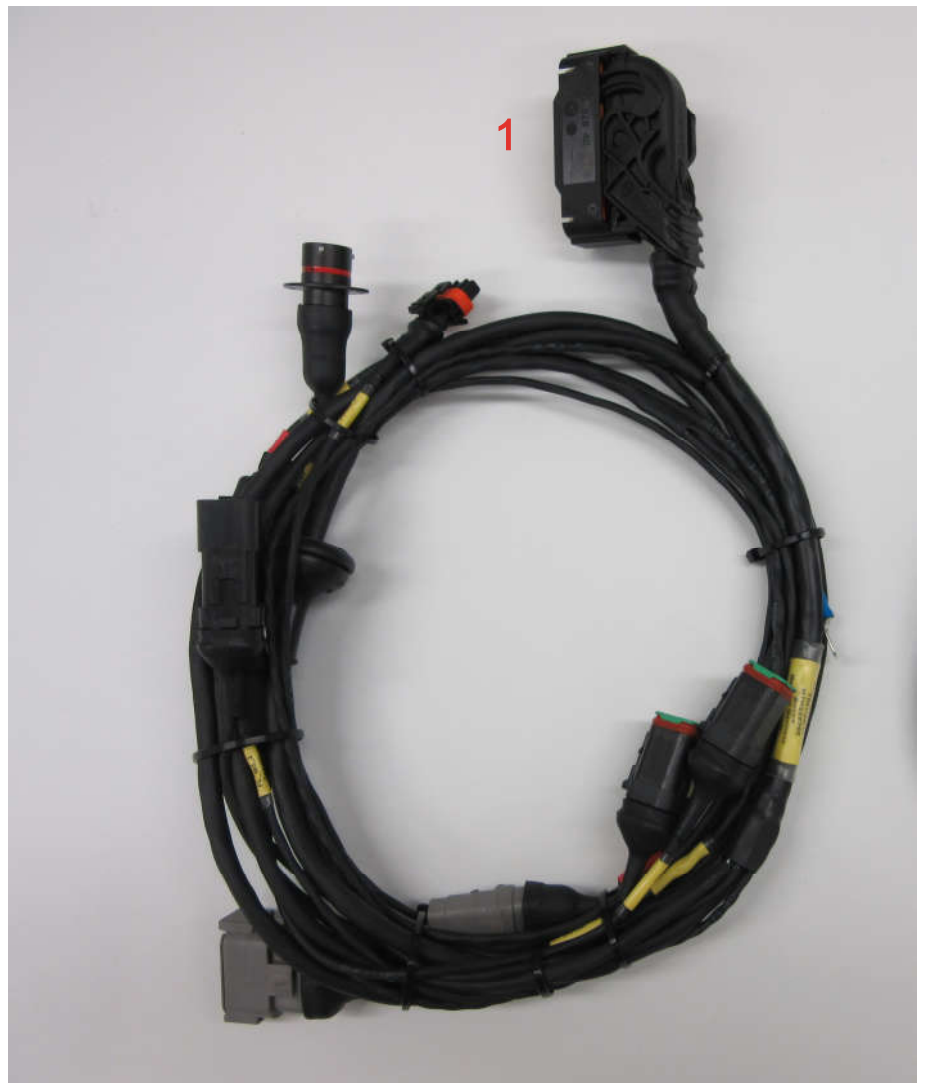
The picture shows the front wire harness with the main connector (1)
