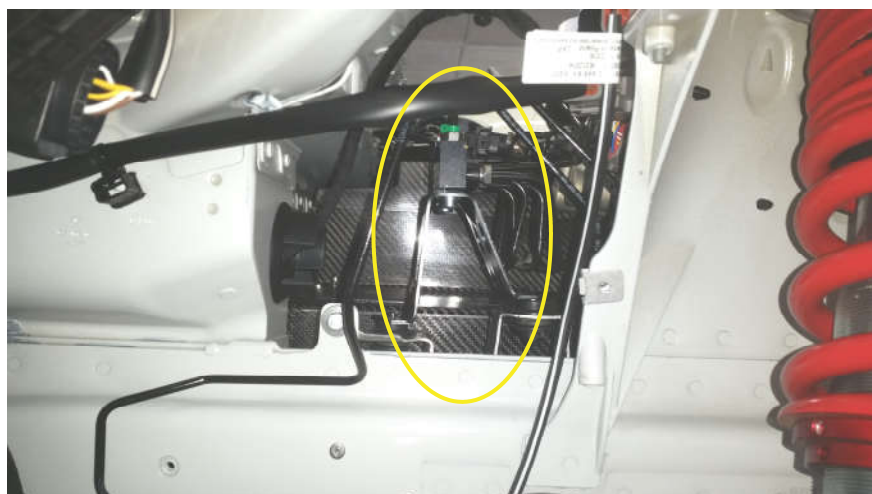
Step 4: Clear view of the line distributor after disassembly of the wheel housing liner
