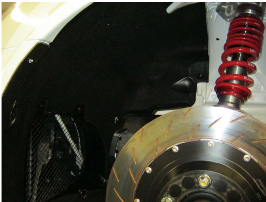
Step 4: Dismantle the front left wheel housing liner
