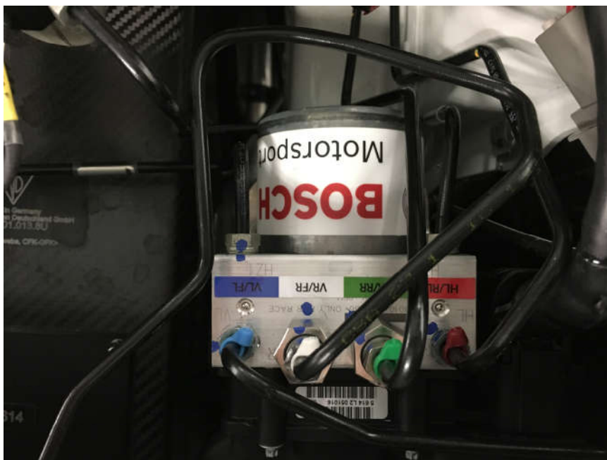
Step 11: Connection of the original brake lines (marked with colored cable ties) to the ABS hydraulic unit
