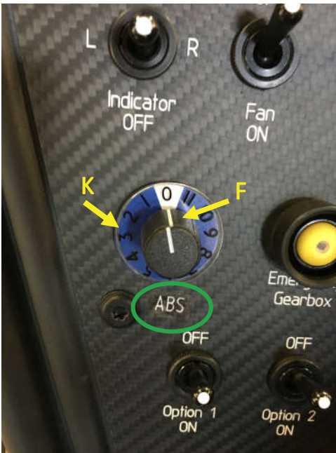
Step 21: Installation of the ABS 12-position switch
