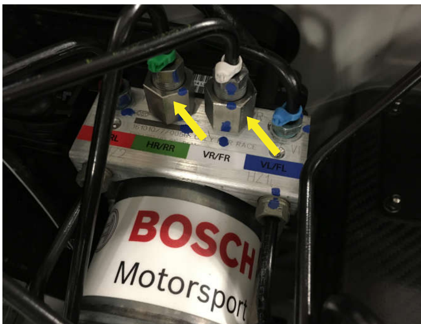
Step 9: Assembly of the new fittings in the outputs (RR) and (FR)
