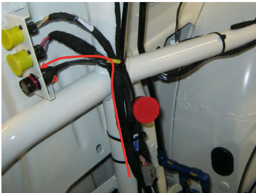
Step 17: Laying and fixing the diagnosis cable
