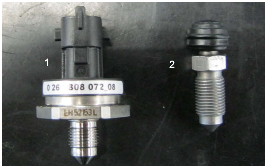
Step 7: New pressure sensor (1) and blanking plug(2)
