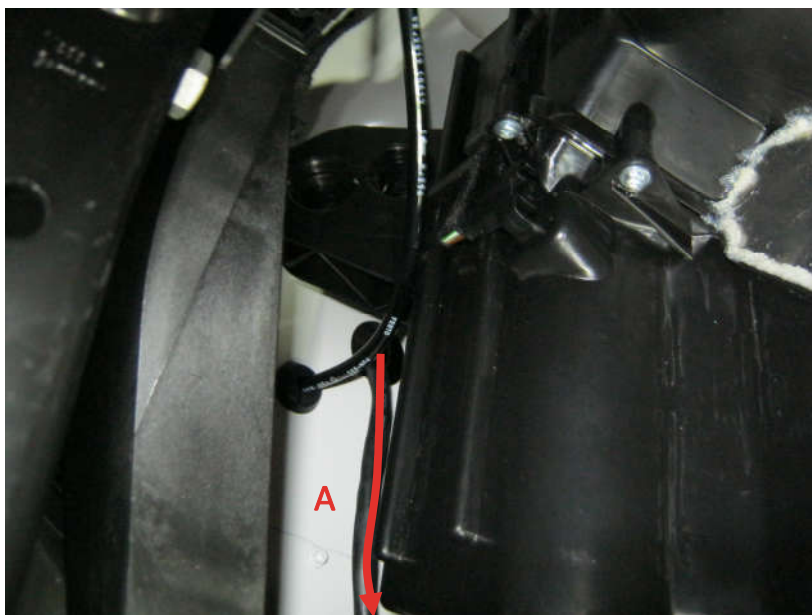
Step 14: Laying the wire harness in the interior (bulkhead)
