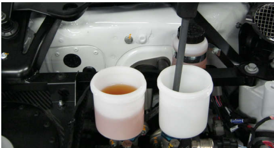
Step 3: Remove the brake fluid from the reservoirs
