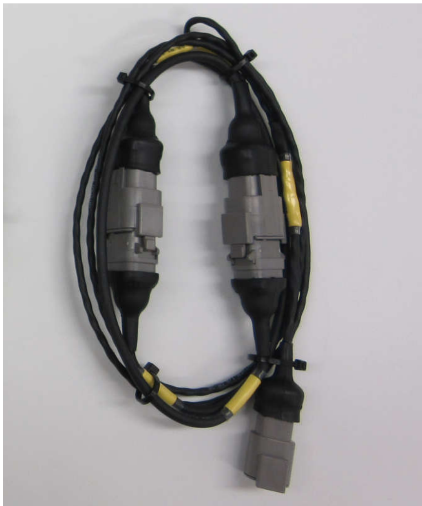
Step 18: rear wire harness for the connection of the wheel speed sensors
