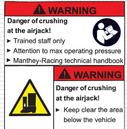
Figure 1.7 Warning Air Lift System
