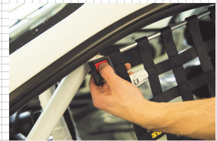
Figure 3.2 The window net can be opened/closed from outside
