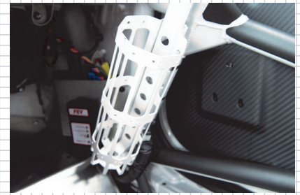
Figure 15.1 Bracket in the area of the A-pillar
