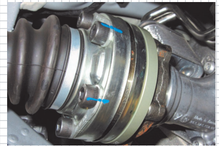
Bild 5.1 Drive shaft spacer between drive shaft and gearbox flange
