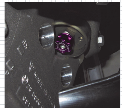
Figure 4.3 Adjustment of the rebound
