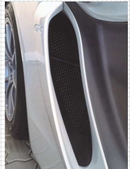
Figure 16.2 Installed Protective Grid.
